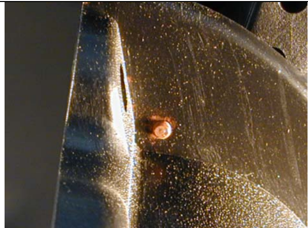
Photo 15 Closing pin oxidation
