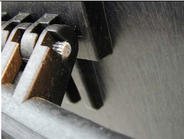
Photo 14 Handle pin oxidation
