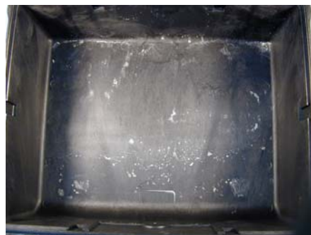
Photo 17 Sample 4820 G – limestone deposit after water steam evaporation
