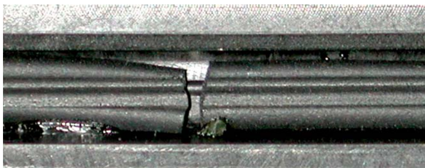
Photo 18 Sample 4820 G – Detail of the separation of the two gasket edges
